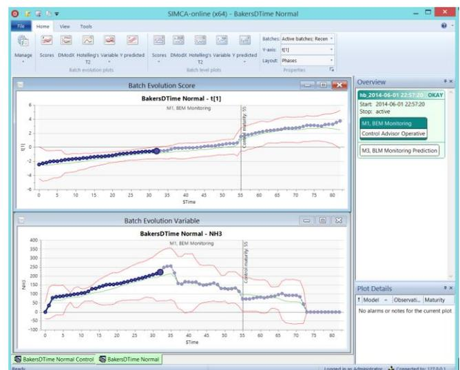
Figure 1. Batch evolution score (top) and univariate (bottom) control charts for Control Advisor in Forecast mode.
